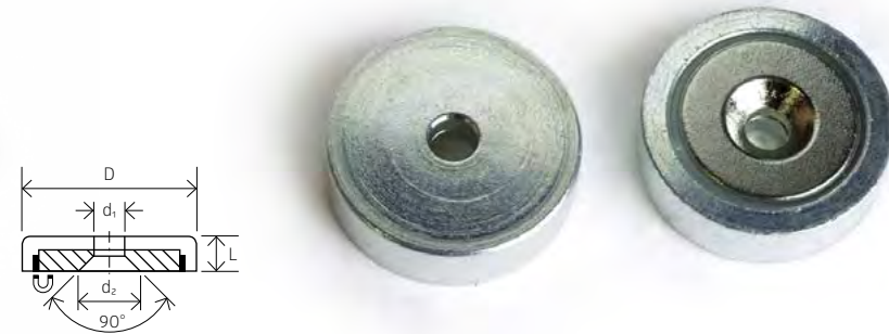
Magnetic system flat, with through borehole and 90° counter bore, magnetic core NdFeB
